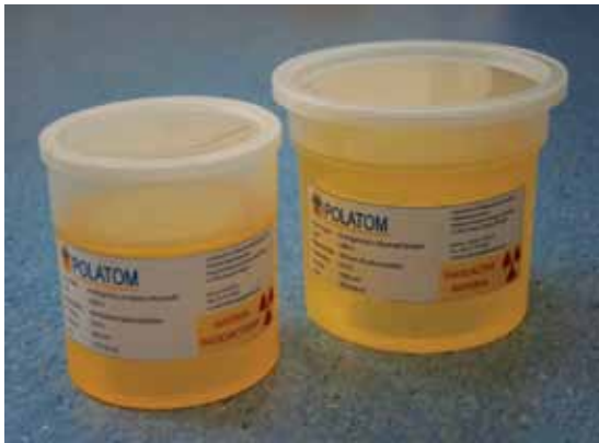
Multigamma sources in epoxy resin.
