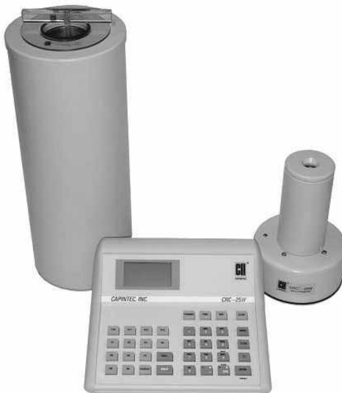
Dose calibrator with 4\pi ionization chamber.
