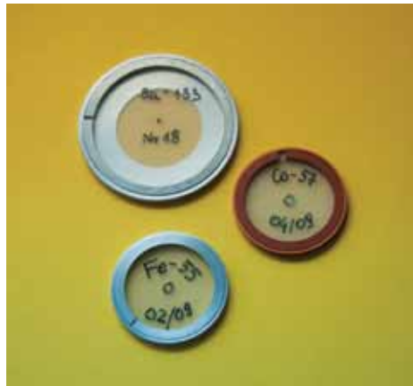
Point sources of \gamma -emitters in polyethylene foil..
