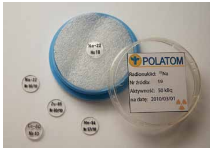
Point sources of \gamma -emitters in Plexiglas.
